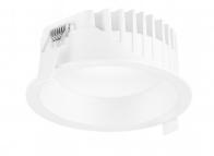
**■ Description**The LILY recessed luminaire has a cast housing, with a PMMA diffuser made as a Fresnel lens shaping the photometric body, resulting in a very low UGR glare in the room. LILY luminaires can be used both in offices, ancillary rooms and to light up communications, entrance halls and toilets.
